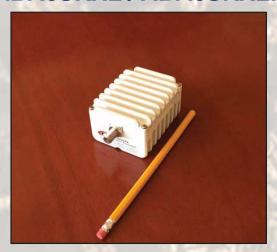
This smallest and lightest 6W L-To Low Ku-Band Block Up Converter is based on GaN technology and is designed to be mounted directly on the feed horn. High power efficiency resulting in low current (< 1 amps @24VDC) consumption allows to use this BUC with any modem without an external power supply.
