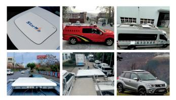
This terminal integrates a fully electronic steering phased array antenna, control unit, up/down converter, and satellite router into a single unit, all housed under one radome. Additionally, it includes wireless access functionality, making deployment easy and efficient. The electronic steering beam ensures high-speed satellite tracking, while the absence of mechanical moving parts guarantees robust reliability.
