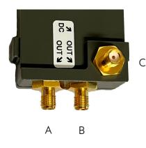
**Connector A** Type: SMA female only Function: RF Output
