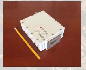
This smallest and lightest 15W L-To X-Band Block Up Converter is based on GaN technology. It is designed to be mounted on the feed horn. High power efficiency resulting in the low current (<2 amps @ 24VDC).
